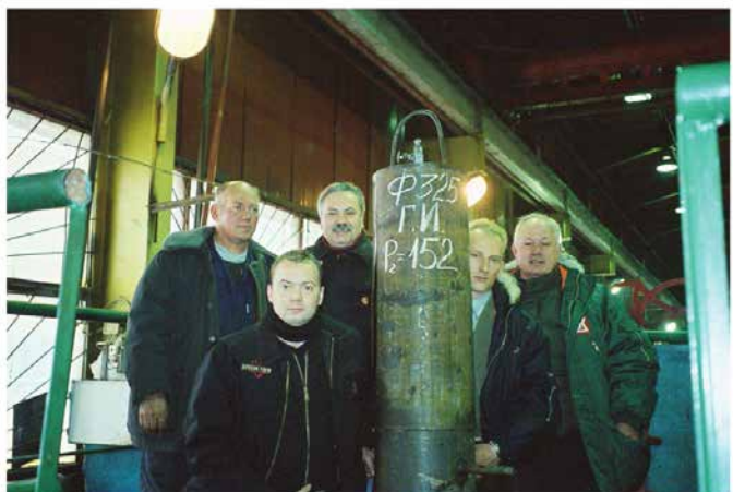
Pressure Test (325mm OD x 8mm Wall) 152 ATM / 2234 PSI
