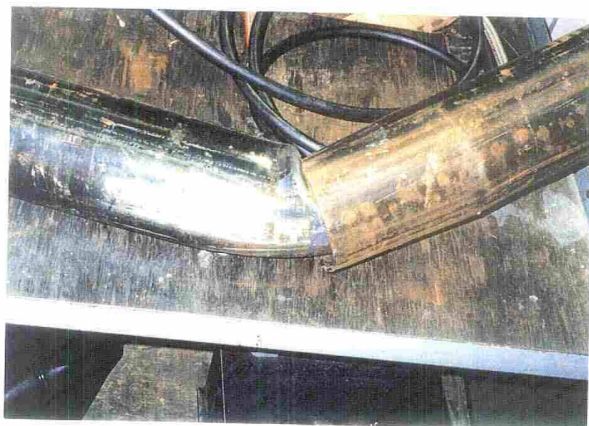
Appearance after Bend Test
